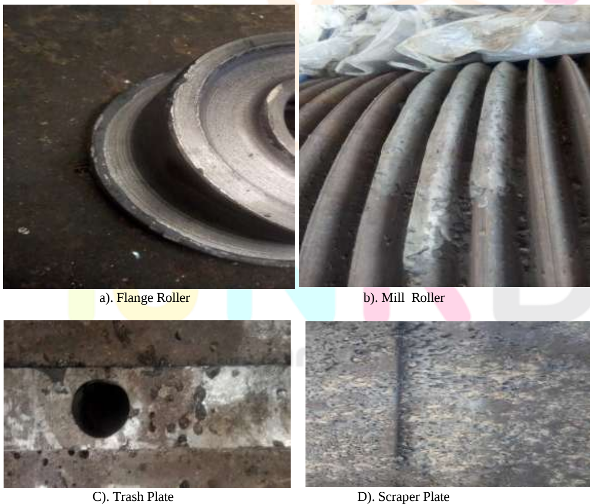
Figure 15: Shrinkage casting defect on different products of precision castings(Observation)
