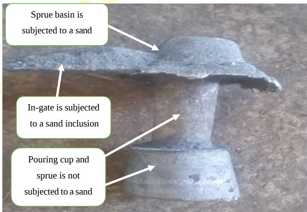
Figure 59: Sand for sprue and pouring cup, good surface finish
