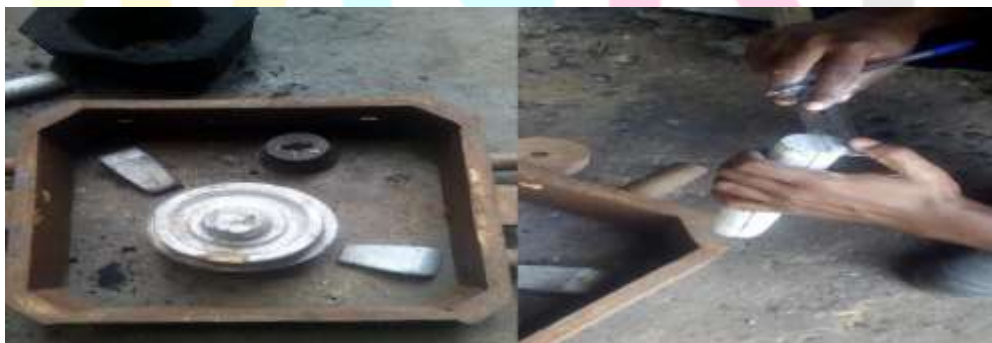
Figure 21: Existing gating system components arrangement (left side), and measuring the gating system components (right side)
