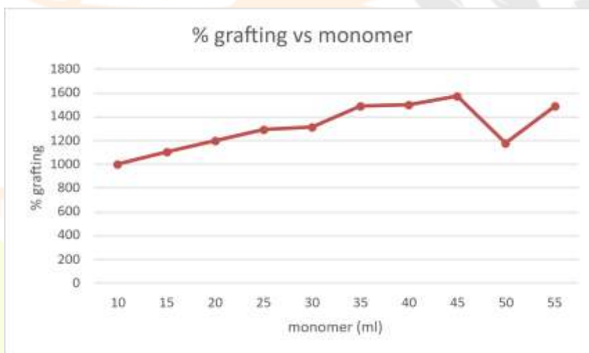
Figure 4.4. Effect of Concentration of Monomer on Percentage Grafting (Pg) of CH-O
