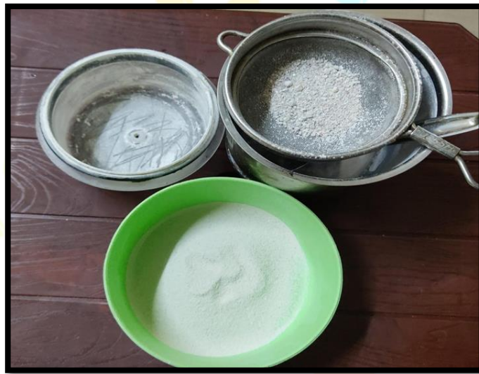
Figure 11,12: Clam and worm shells were ground using a 600W personal blender
