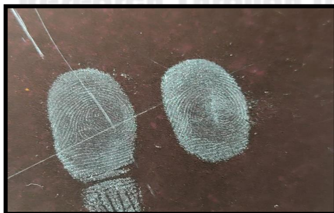
Figure 20: Finger print developed on the wood surface
