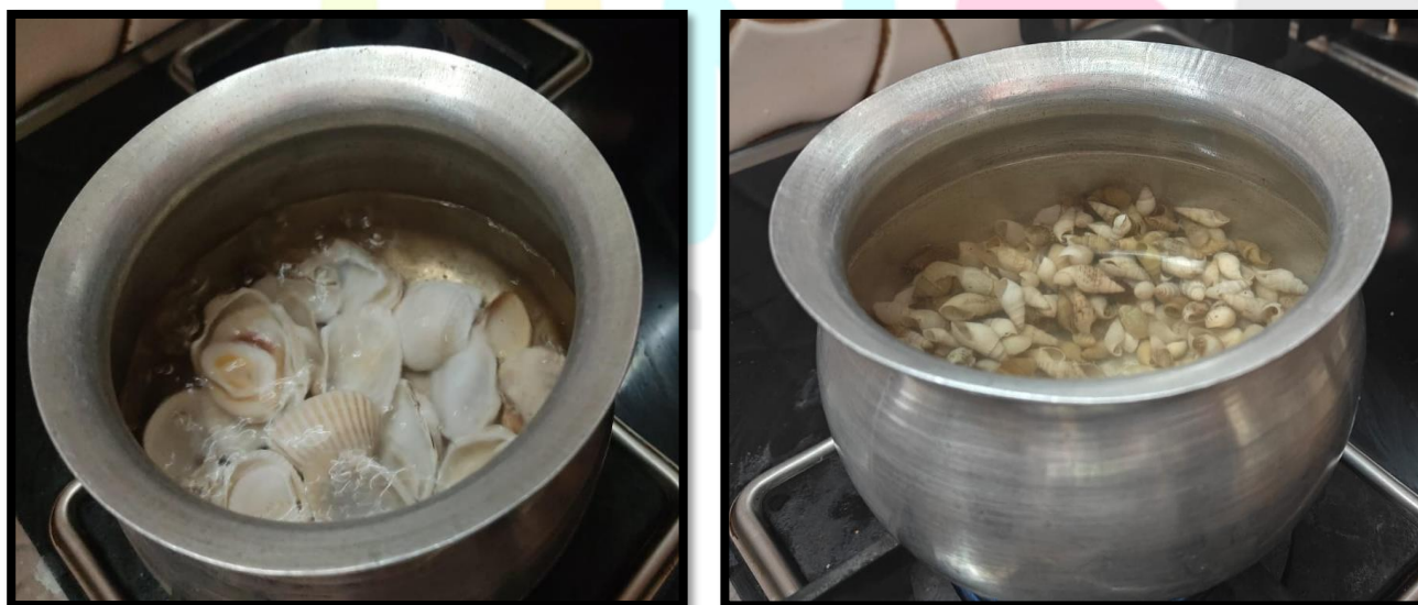
Figure 7, 8: The collected clam and worm shells were boiled in distilled water
