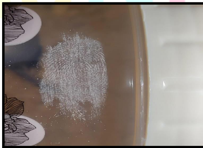
Figure 17 : Finger print developed on the Plastic Surface
