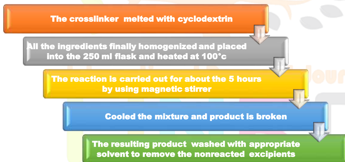
Figure 5 Schematic Representation of Melt Method.
