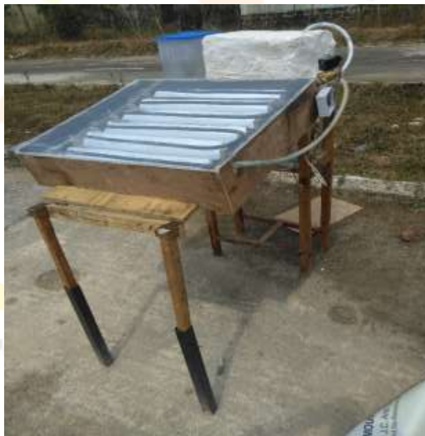
Figure B10: Fabricated solar water heater with thermal energy collector
