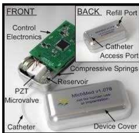
Fig 1- A photo of the front of an assembled microvalve regulated drug delivery device with the back side refill port shown inset
