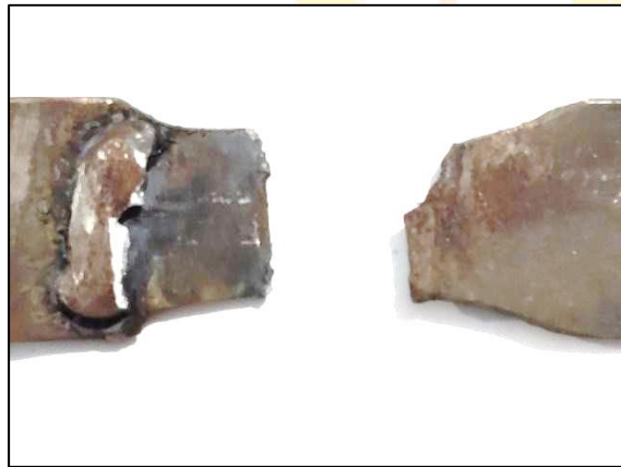
Fig2(c) Sample -3 post tensile test with 2.5 - mm electrode, currents of 260 Amps
