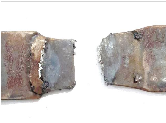
Fig3(a). Sample- 5 post tensile test with 4- mm electrode, currents of 240 Amps
