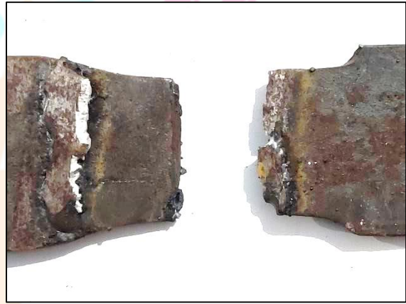
Fig2(d). Sample -4 post tensile test with 2.5- mm electrode 2.5mm electrode, currents of 270 Amps
