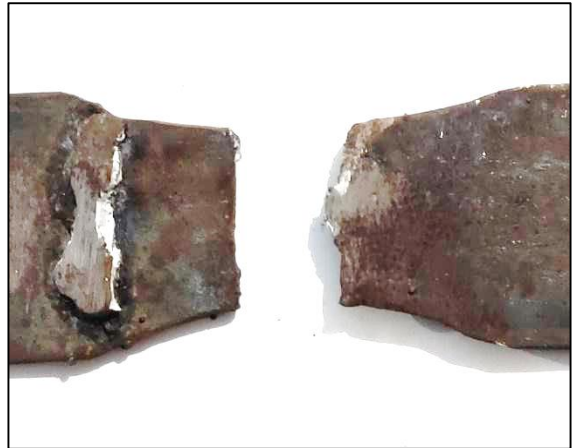
Fig 2 (b). Sample- 2 post tensile test with 2.5mm electrode currents of 250 Amps
