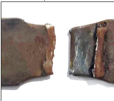
Fig2(c) Sample -3 post tensile test with 2.5 - mm electrode, currents of 260 Amps
