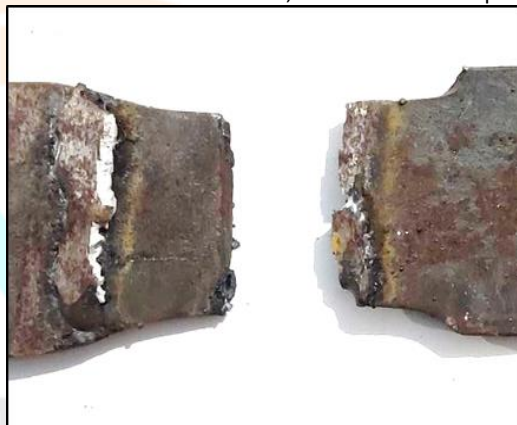
Fig2(d). Sample -4 post tensile test with 2.5- mm electrode 2.5mm electrode, currents of 270 Amps
