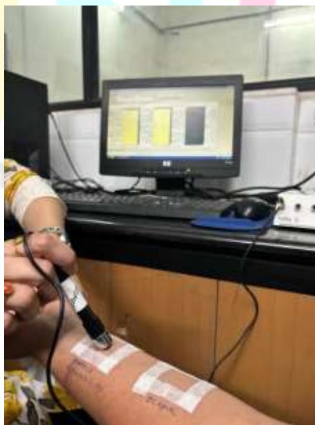
Fig.6 - Moisture measurement of Skin by Corneometer
