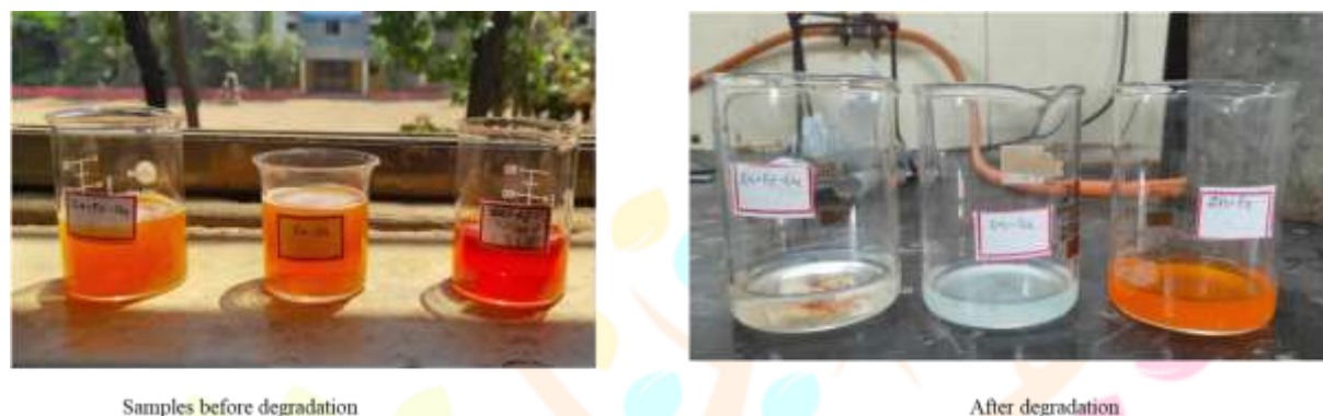
Figure 7: Samples before and after dye degradation study
