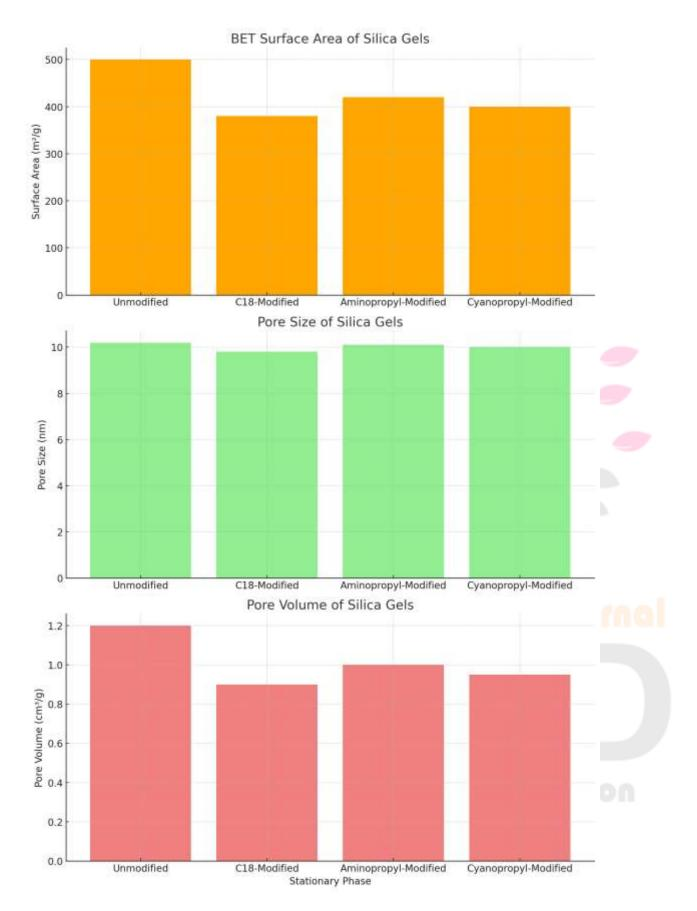
**Interpretation**: The reduction in surface area for the modified gels compared to the unmodified silica is consistent with the successful attachment of functional groups, which occupy surface sites. The pore size and pore volume decrease slightly, indicating that the modifications affect the porosity of the stationary phases.
