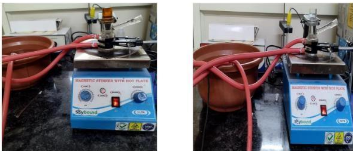
Figure 12: In-vitro Dissolution study diffusion cell
