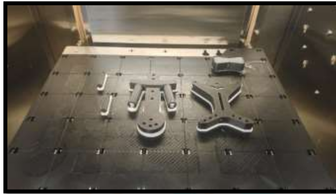
FIGURE: 3 (3D Printing of joint in Stratasys F370 printer)
