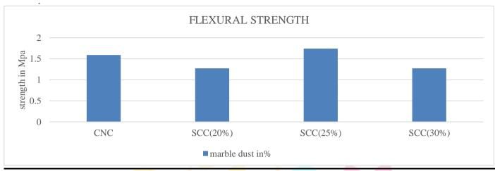
This indicates that the addition of 25% marble dust has significantly improved the flexural strength of the concrete at 28 days, outperforming all other mix ratios by a margin of 10%
