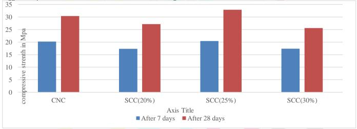
From the table 5.2 it is observed that the compression test at 7 & 28 days result 20.22 N/mm2 & 30.35 N/mm2 respectively 25 percentage inclusion of marble dust which is greater than 2% for 7 days & 8% for 28 days compare to all mix ratio of concrete.
