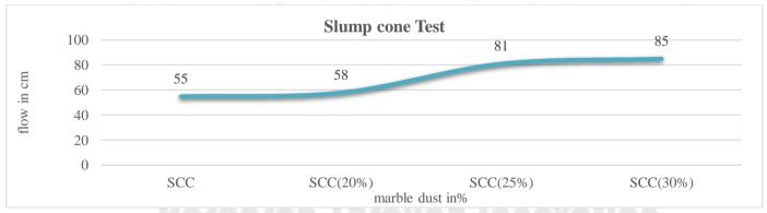
Self-Consolidating Concrete (SCC) with a 25% mix design exhibited:
