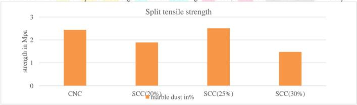
From the table 5.4 it is observed that the split tensile test at 28 days is 2.44 N/ mm2 at 25 percentage inclusion of marble dust which is greater than 3% compare to all mix ratio of concrete.
