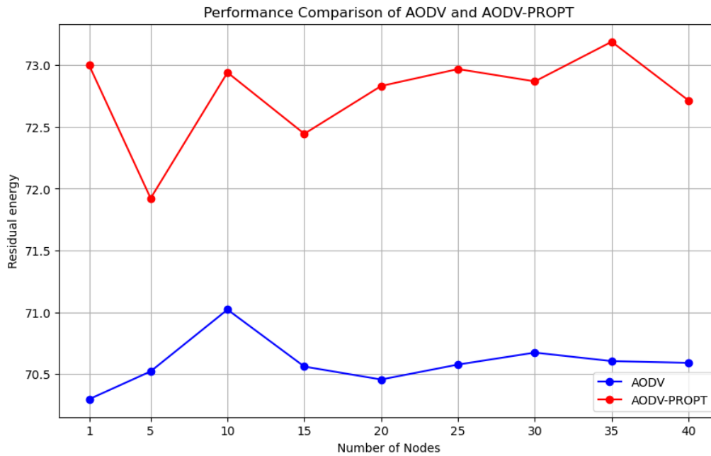
Fig 10: Line graph comparing residual energies values for 40 nodes
