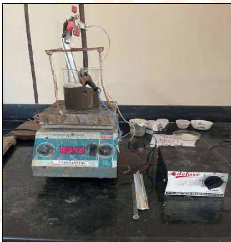
Fig 1: Experimental setup of electro- coagulation treatment
