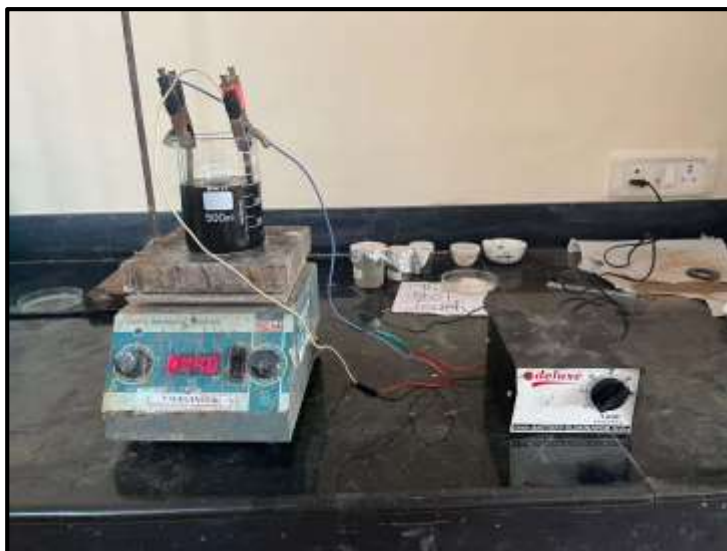
Fig 2: Experimental setup of Electro-Fenton setup
