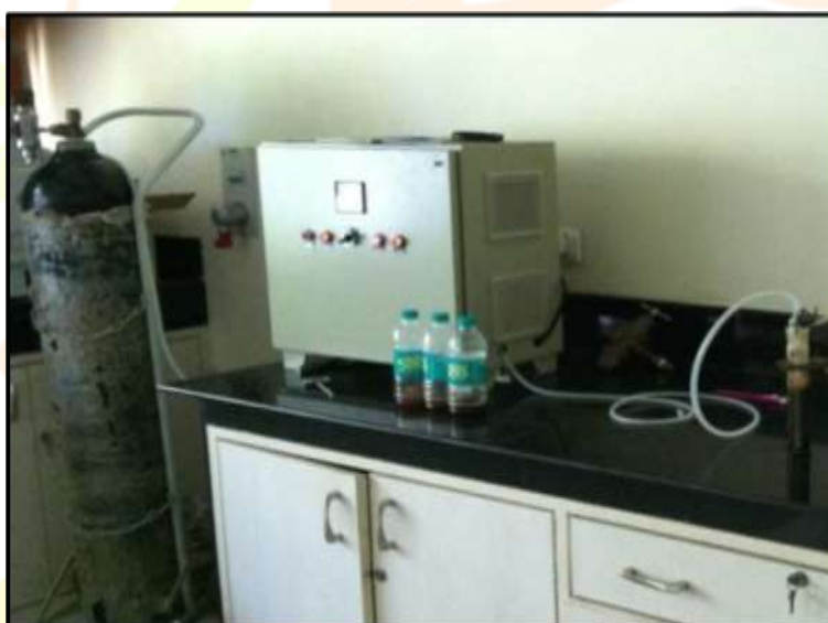
Fig 3: Experimental set up of the ozonation treatment
