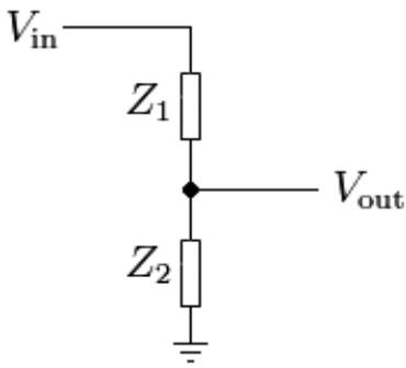
Fig Voltage divider
