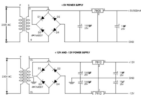
Fig Circuit diagram for Regulators
