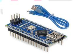
**Prototyping**: Arduino Nano boards are often used for prototyping electronic circuits and systems. Their small form
