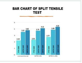
**BAR CHART OF TABLE 3:** As per the above bar chart the split tensile strength of concrete goes on increasing with the increment of steel fibers.
