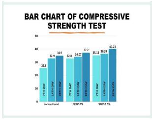
bar chart the compressive strength of concrete goes on increasing with the increment of steel fibers.
