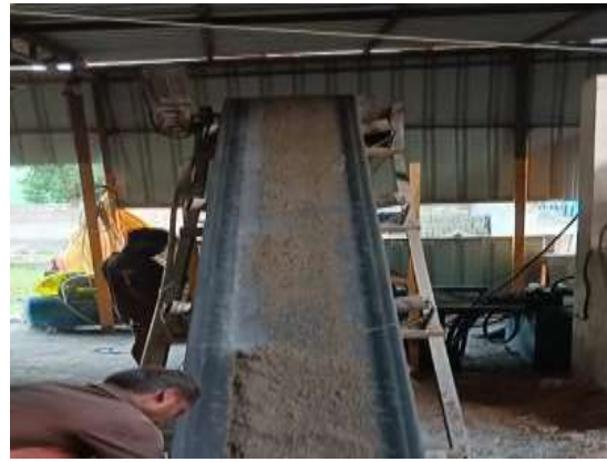
Fig 5.4 It is then compressed to form bricks with desirable interlocking patterns when the required mix is prepared.
