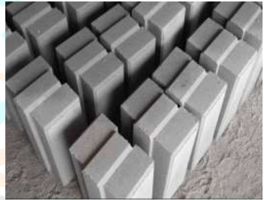
Fig 5.6 Then for about 7 days, these bricks are subjected to wet curing and next days dry curing
