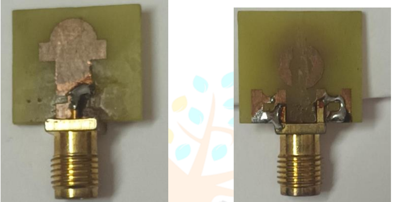
fig2.8: Hardware implementation of the proposed antenna
