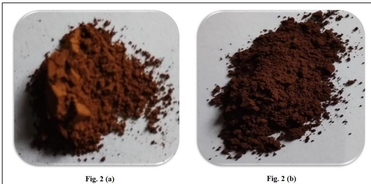
Fig. 3 (a) and Fig. 3 (b) shows the synthesized \text{BiFeO}_3 powder samples using glycine fuel and urea fuel
