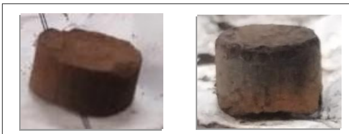
Fig. 4 (a) and Fig. 4 (b) shows the pellets of prepared \text{BiFeO}_3 powder samples using glycine fuel and urea fuel
