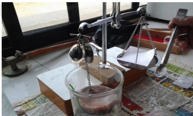
Fig. 2: Modified physical balance for determination of bioadhesive strength
