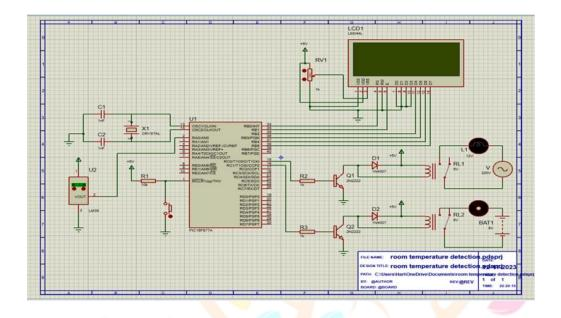
Figure.04: Temperature system simulation circuit
