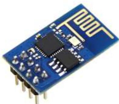
The ESP-01 has 8 pins, including 2 GPIO pins. - Antenna on a PCB trace. (As in the figure above)
