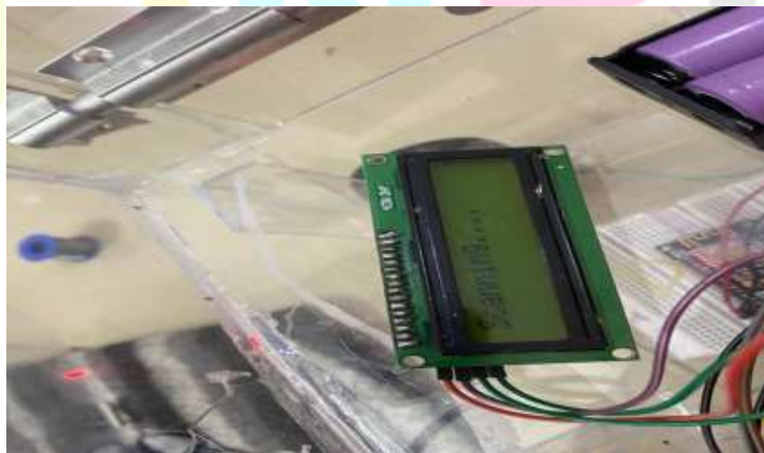
Figure.5. display shows scanning when we put the rfid card
