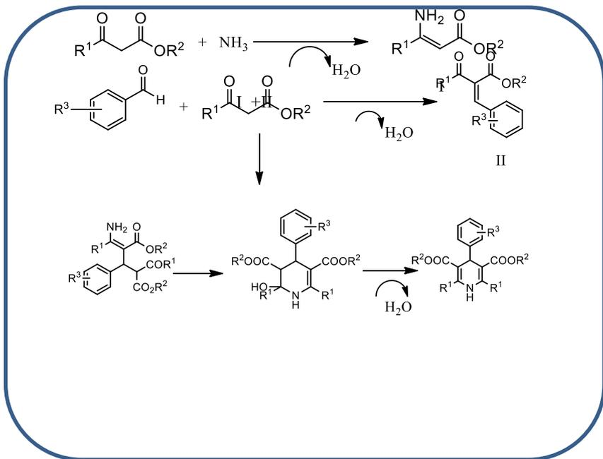
**SCHEME: 2, Mechanistic pathway for the synthesis of Hantzsch Dihydropyridine**
