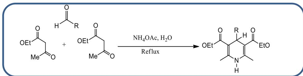
**SCHEME: 1, Synthesis of Dihydropyridine.in aqueous medium**
