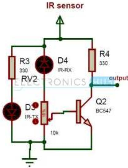
Fig.2.IR sensor equivalent circuit
