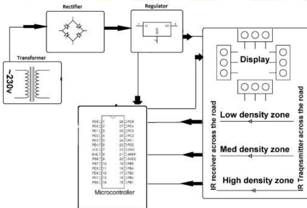
Fig1. Block Diagram of signal control system
