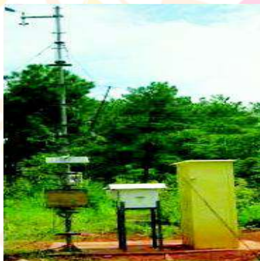
Fig.6: Fuel cell AWS installed by ISRO at Shillong [27]
