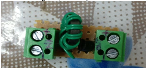
Fig (viii): Joule thief circuit on PCB
