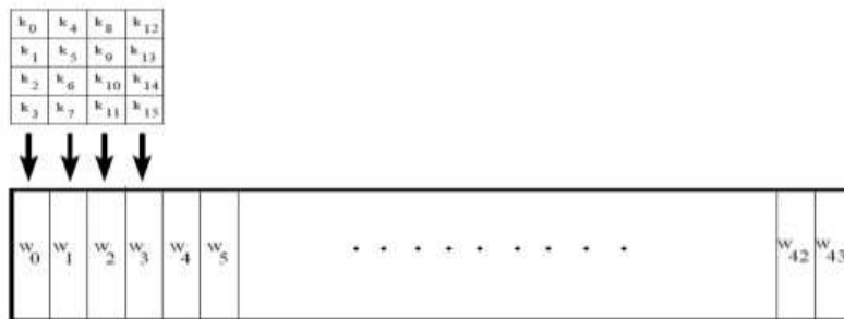
Fig -7 This figure shows the four words of the original 128-bit key being expanded into a key schedule consisting of 44 words.
