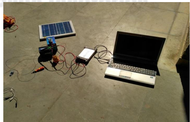
Fig. 8. Charging of Battery without MPPT by 15 Watt Panel
