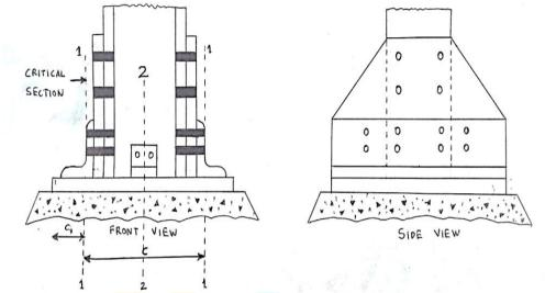
The function and purpose of column base plates are to provide a spread and distribution of column loads from the steel column to the concrete footing. In short, the base plate acts as an intermediate stress distributor. When the column load contains a moment, the base plate may require to design in such a way that to ensure uplift of the base plate does not occur, and which will be achieved by designing anchor bolts to resist the tensile forces.
